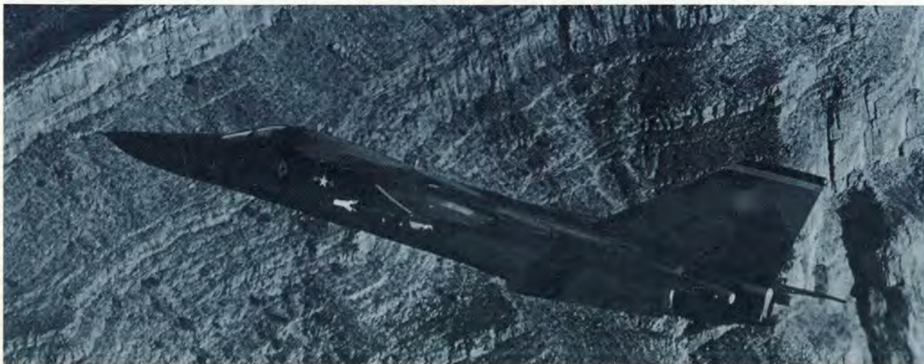
The F-111 is a tactical strike aircraft that can fly at supersonic speeds and operate from tree-top level to altitudes above 60,000 feet.
